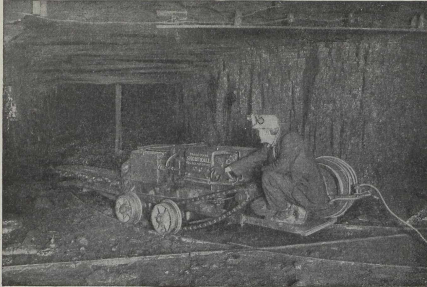
Figure 1. Illustrating the method in which the machine enters the room on its own truck
