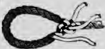
Fig. 3—Beginning the Eye-Splice.
