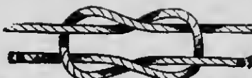
Fig. 5—Upper Diagram shows the Granny Knot; the center, the Square or Reef Knot, and the lower, the Thief Knot. The Granny and Thief Knots are worthless.
