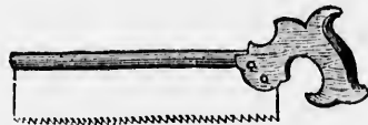
Meat Saw, for sawing bones in parts of meat where the chopper cannot be used.
