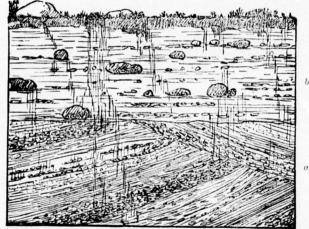
1. Section of Drift on Milk River-(a) Boulder-clay; (b) older river alluvium; (c) newer
