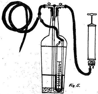
Fig. 5.—Aspirator with manometer attachment for relief of tension pneumothorax.
