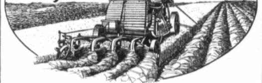
The advantage of the wide drive drum as used in Gray Tractor is greater traction surface and the elimination of soil packing, the weight being distributed over a large surface. Packers or disks attached to the side arms with a 26-ft. drag, will prepare 60 acres of seed bed in a ten-hour day.
