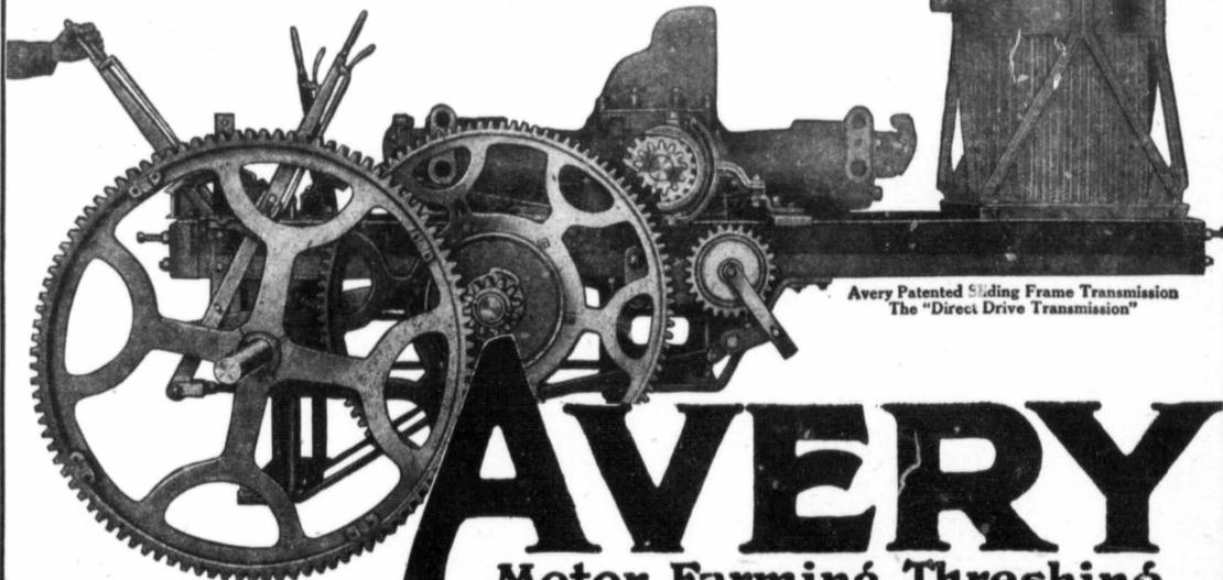
Avery Patented Sliding Frame Transmission The "Direct Drive Transmission"
