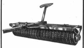
The Western Pulverizer, Packer and Mulcher pulverizes and packs down the soil and puts it in perfect condition for seeding in one operation, either a stubble ground or sod ground. It will not clog. Provides a granular mulch to the land which stops evaporation and preserves moisture.
