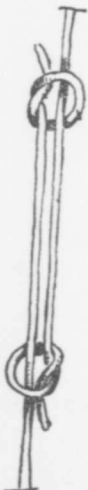
The fisherman's knot. It never slips; is easily opened by pulling the two short ends.
