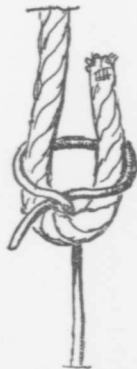
Becket hitch, for joining a cord and a rope.
