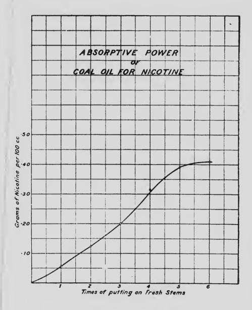
of nicotine in the oil and its rate of passage through the approratus. An extractor 2 centimetres in diameter and 40 eer imetres long, containing twelve baffle plates removed all the nicoune from a solution containing 0.2 grams per 100 cubic centimetres, when passed at the rate of 25 cubic centimetres per minute. Another effective method was to spray the oil solution into the acid, under pressure, through a fine nozzle.
