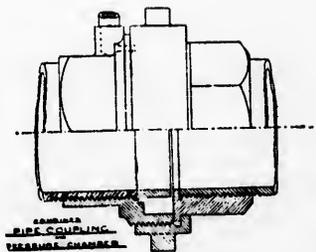
diameters and 10 of four diameters. At the central cross-section of each bend, provision is also made for ascertaining the pressure, either by a mercury column or by a gauge, at the extremities of the radii to the outer and inner surfaces of the bore. The chambers for the bonds are combined with union couplings, of the same bore, which allow the attached part to be swivelled through any required angle.
