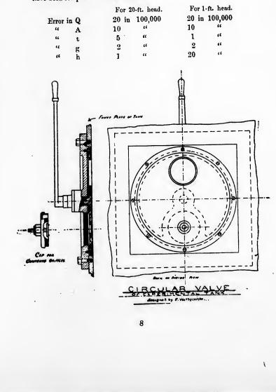
Perhaps the most important feature of the tank is the valve arrangement. The valve is a gun-metal disc 3-in. in thickness and 24-ins. in diameter, fitted into a recess of the same dimensions in a cast iron cover plate, with gun metal bearing faces, forming a water-tight joint for the face of the disc. This cover place or body is bolted to an opening in the front of the tank, and the inner faces of the cover plate or disc are flush with the inner surface of the tank.
