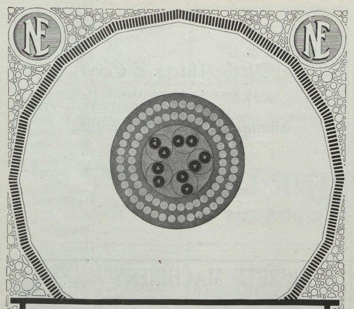
5 Pair No. 16 B. & S. Rubber Insulated Double Steel Wire Armored Submarine Telephone Cable
