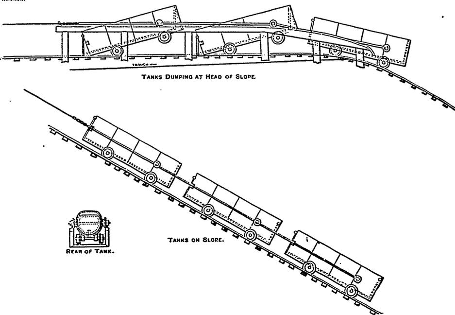
FIG. 1.—Self-Loading and Self-Dumping Water-Tanks.
