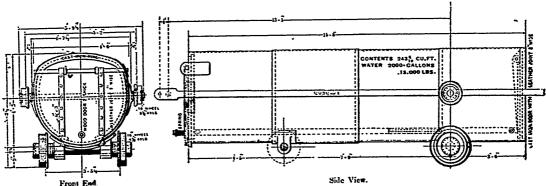
bearings while the tanks are immersed, and to retain the lubricant. Each tank is provided also with side-wheels, vertically over the rear axle, which have a guage sufficiently wide to clear all other portions of the tank; and on the surface an elevated track is provided, upon which the dumping wheels run and thus raise the rear end of each tank as much as may be necessary to dump the water into a trough between the tracks; the tilting for-
