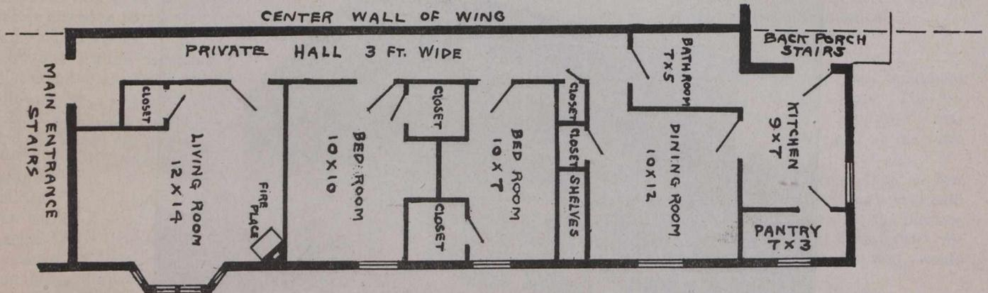
Sketch showing typical floor plan of five-room suite with private hallway. Solid fire wall dividing wing of building is shown.
