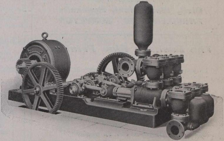
Horizontal Treble Ram Pump, driven by Electric Motor
