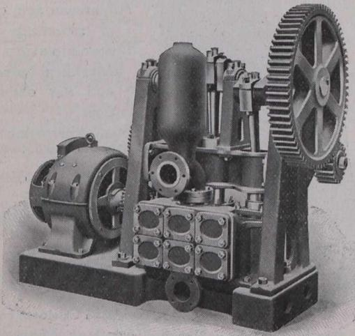
Vertical Treble Ram Pump, driven by Electric Motor
