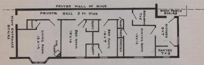
Sketch showing typical floor plan of five-room suite with private hallway. Solid fire wall dividing wing of building
