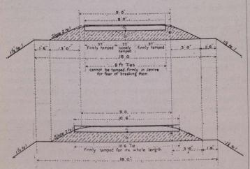
Note.—8-ft. ties tamped firmly for 16-in. each way from rails only utilize the supporting area of 77 per cent. of tie, equal to 74-in. in length, or 740 square inches for a tie of 10-in. face.
