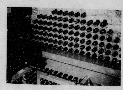
A remotely controlled fueling machine, positioned at the reactor face. Fuel bundles are changed while the reactor remains "on power."
