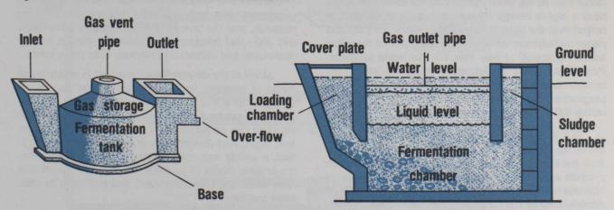
Figure 6-6: CHINESE DESIGN OF A BIOGAS DIGESTER
