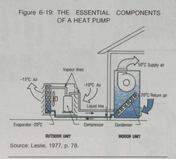
absorbs heat, its latent heat of vaporization, from the surrounding air which is in turn cooled somewhat by the process. A compressor circulates the gas back to the building where it is condensed and changes state back to a liquid, giving up its latent heat of vaporization and warming the interior air.
