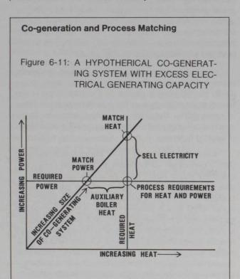
The illustration above represents a co-generation scheme where the ratio of power to heat exceeds that required at the site. The sloped line beginning at the origin and rising to the right represents a co-generating system of increasing size. Reflecting the power/heat ratio, the slope of the line is characteristic of the system in question and is a function of the temperature at which heat is required in the process.
