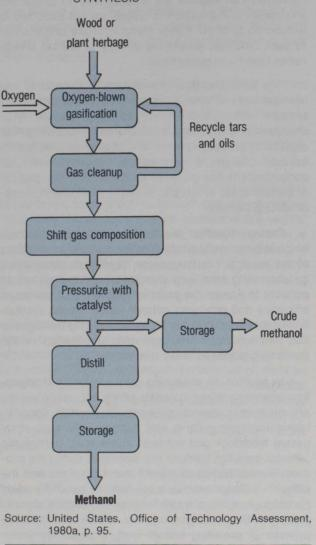
Figure 6-5: PROCESS DIAGRAM FOR METHANOL SYNTHESIS
