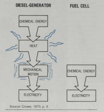
water. Fuel cells of the *direct* type utilize pure  $H_2$  and  $O_2$  which have been produced independently whereas cells of the *indirect* type are combined with a hydrogen-generating unit which can produce hydrogen from a wide variety of fuels.
