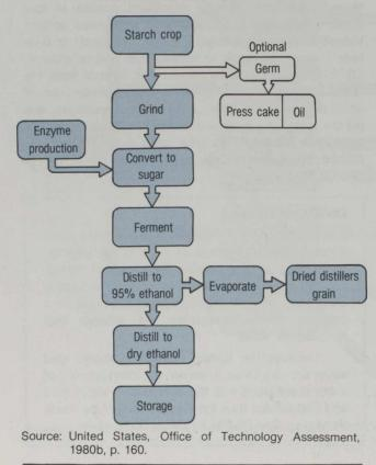
Figure 6-3: PROCESS DIAGRAM FOR THE PRODUC-TION OF FUEL ETHANOL FROM STARCH-CONTAINING CROPS
