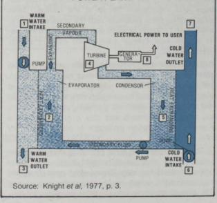
sent up to half the total plant investment) and the exchangers themselves present a continuous problem with corrosion and fouling with marine creatures on their seawater side.
