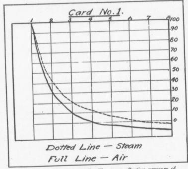
or otherwise a later cut off. The mean effective pressure of the air in this case is 41.6 and the steam 33.46, but the volume of air used is .2353 and the volume of steam used is .1473, the saving in the use of steam here is 25 per cent.
