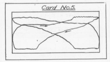
cylinder to be again compressed with an additional temperature perhaps high enough to ignite. As a remedy for this, the discharge valves should be cleaned often and only the best oil used for lubricating the air cylinder.
