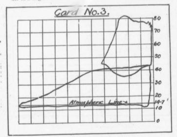
Here you will experience another loss by using an intercooler that is too small. Card 3 is a rough card which will show this. The depressed inlet curve of the second stage card shows this loss which is due to the small area of the intercooler and to the shrinkage of volume in it caused by cooling and causing a loss in the second cylinder. With cooling receivers of the proper capacity this loss would not be. Card 4 shows the economy of two stage compressors to 100 pounds.
