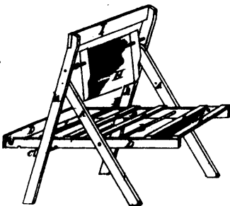
8473 Barlow, Terrill and Taylor's Machine for Holding Wash Tubs.
