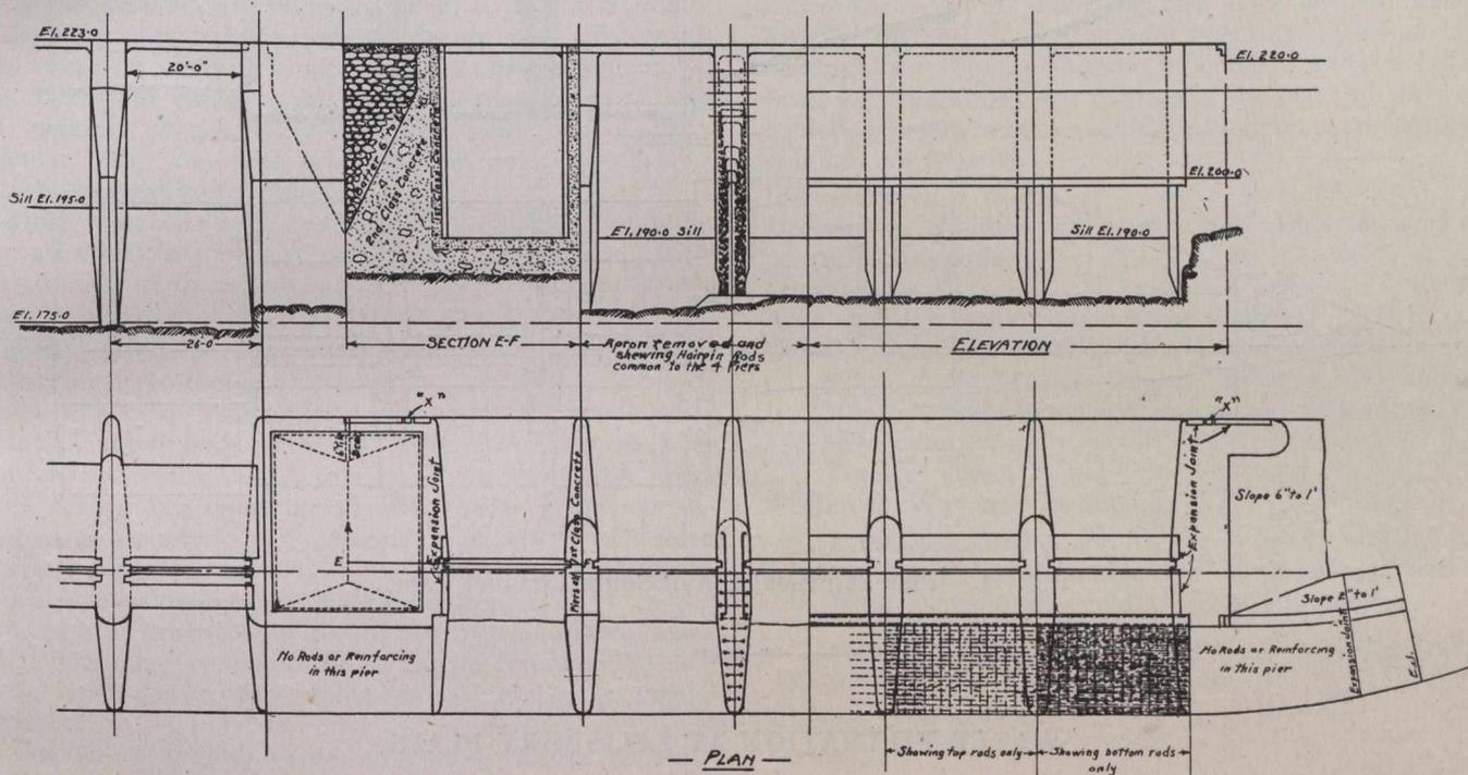
Fig. 10.—Plan and Elevation of Governing Dam.
