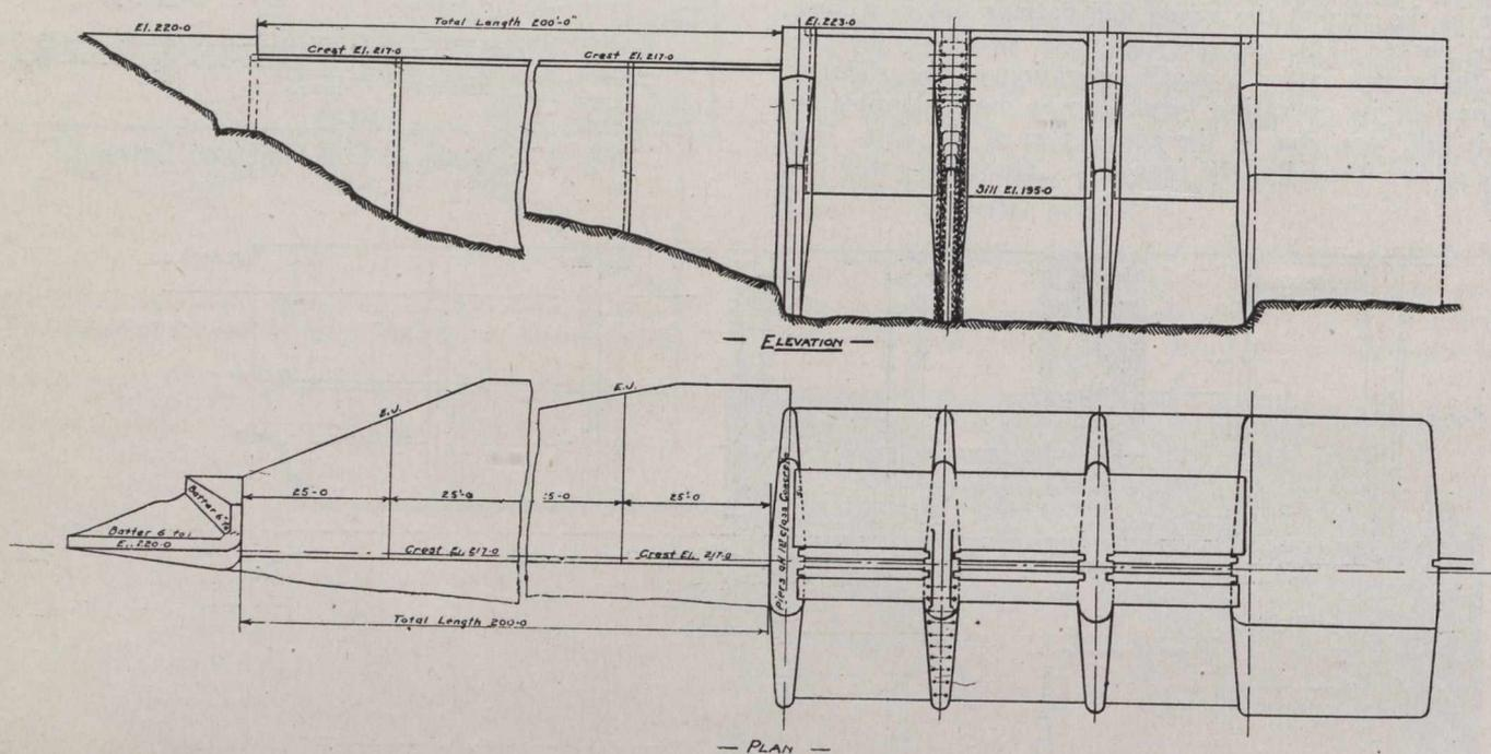
Fig. 11.—Plan and Elevation of South Channel Dam.
