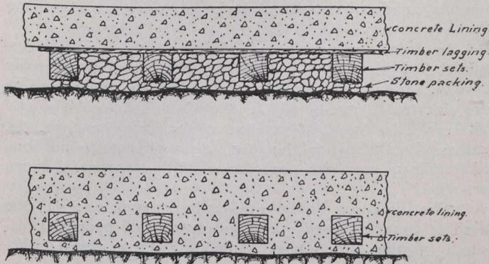
Fig. 5.—Horizontal Sections Through Side-wall of Tunnel Illustrating Two Different Methods of Construction.
