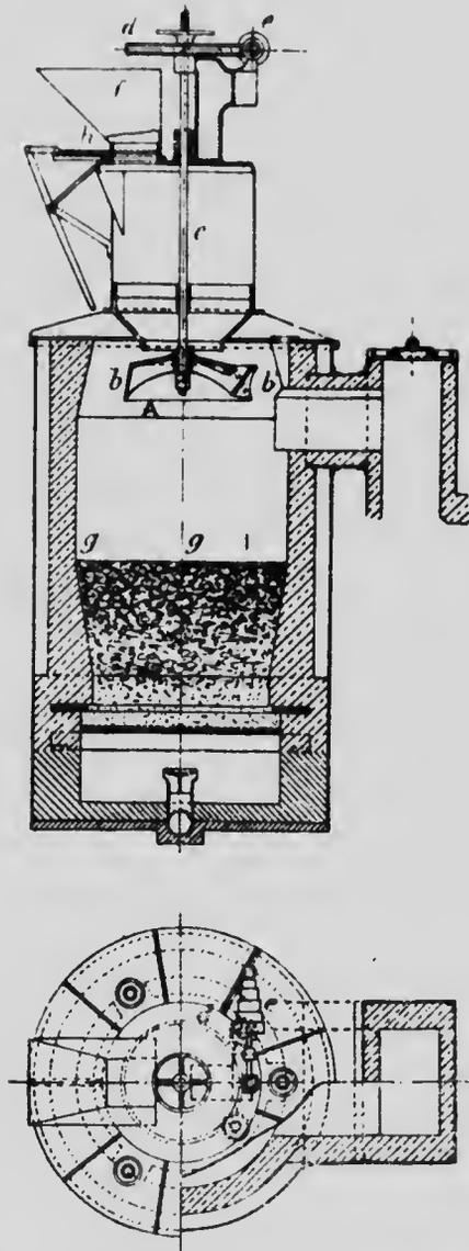
FIG. 194 W. Bildt's Producer with Automatic Feed Device.
