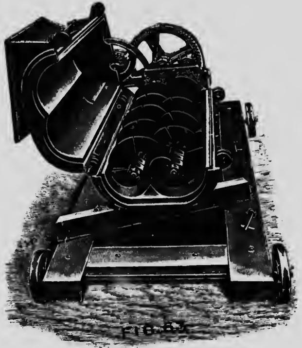
FIG. 63—R. Dolberg's Peat Machine No. 1a (interior).
