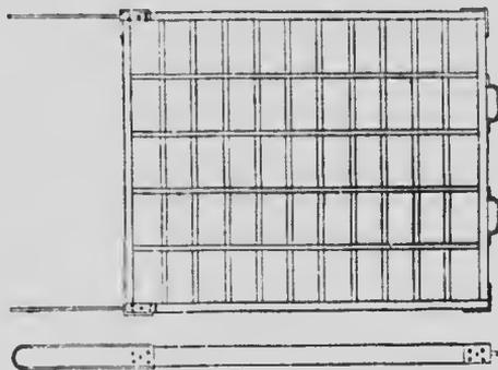
Fig. 37 Peat Moulds used at Ökaer.
