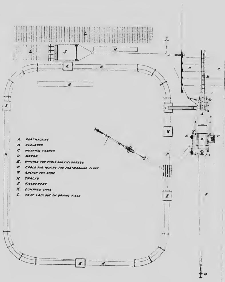
FIG. 114.—Anrep Svedala Peat Plant with cable transportation on round track and fieldpress.
