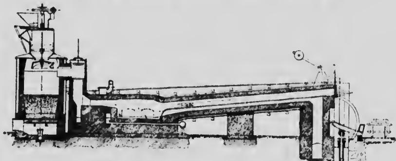
FIG. 195—Bildt's Producer combined with Re-heating Furnace.
