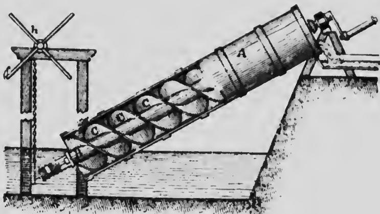
FIG. 1. Closed Water-screw.
