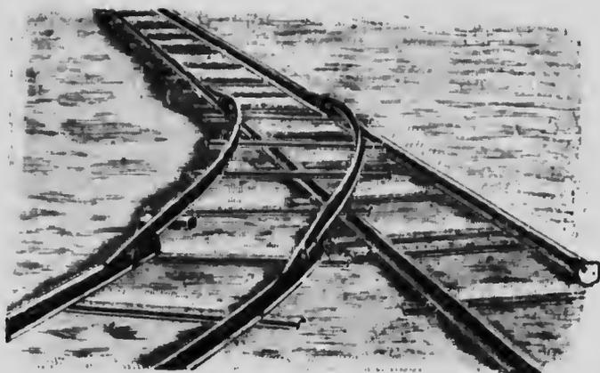
FIG. 38—Portable Curve.
