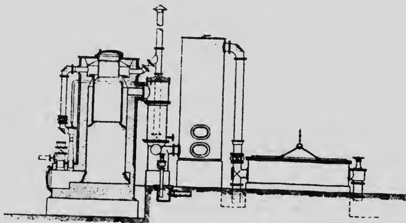
FIG. 203—Pintsch Gas-producer for Bituminous Fuels.
