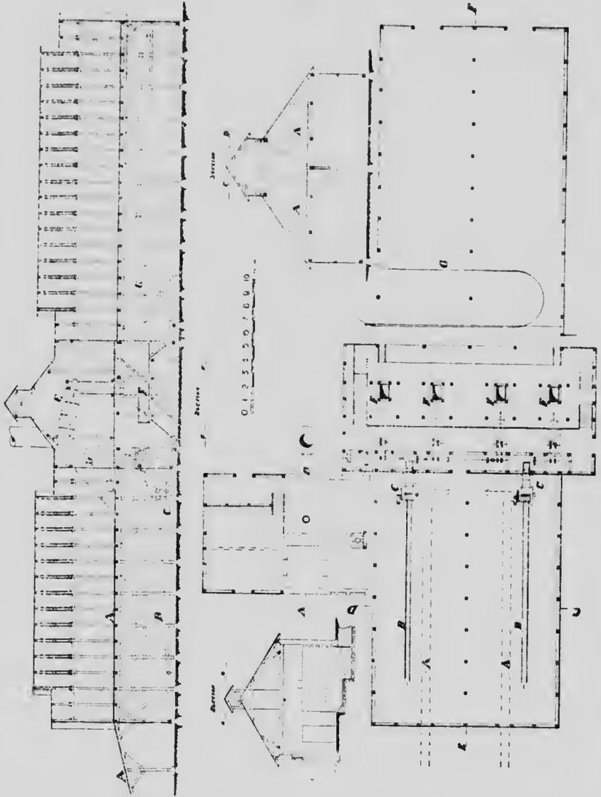
FIG. 227.—Moss Litter Plant with Four Presses.
