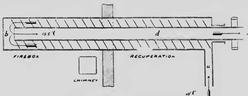
FIG. 171—Theoretical working of a Wet Carbonizing Oven.
