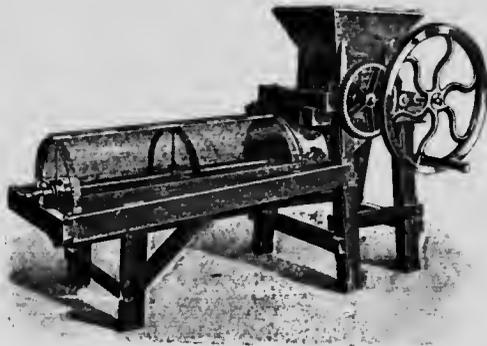
FIG. 215—A. Heinen's Moss Litter Disintegrator for Hand-power.
