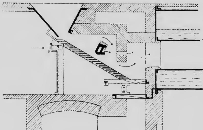
FIG. 189—Keilmann & Völcker's Half-gas Furnace.
