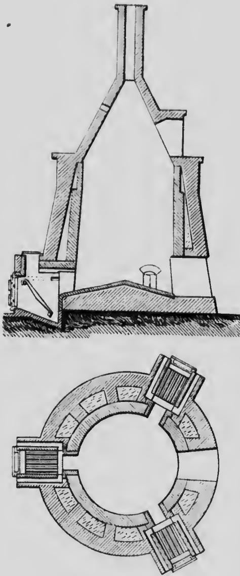
FIG. 197—Lime Kiln with Half-gas Firing.
