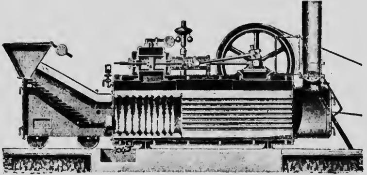
FIG. 185—Locomotive with Step-grate, from H. Lantz, Mannheim, Germany.
