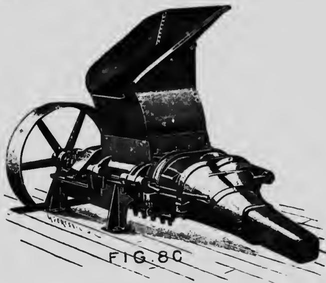
FIG. 80. Anrep's Peat Machine with two shafts (exterior).
