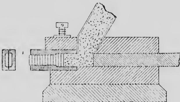
FIG. 155—Section of Briquette Press.
