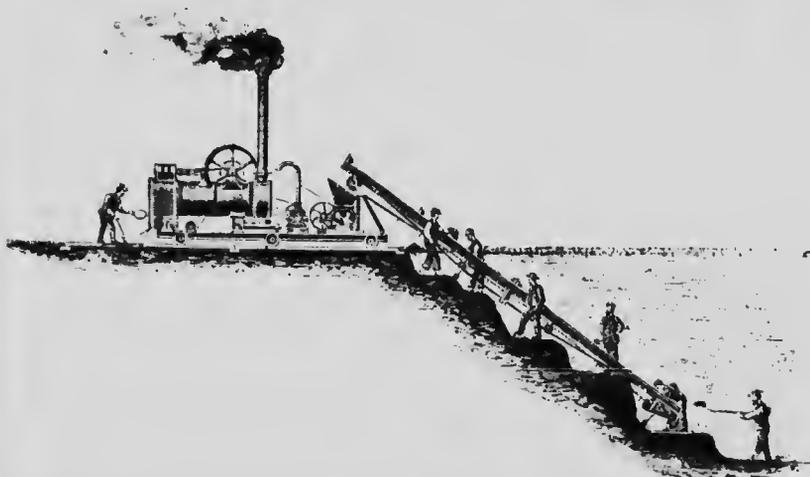
FIG. 69—R. Dolberg's Peat Plant with end elevator.
