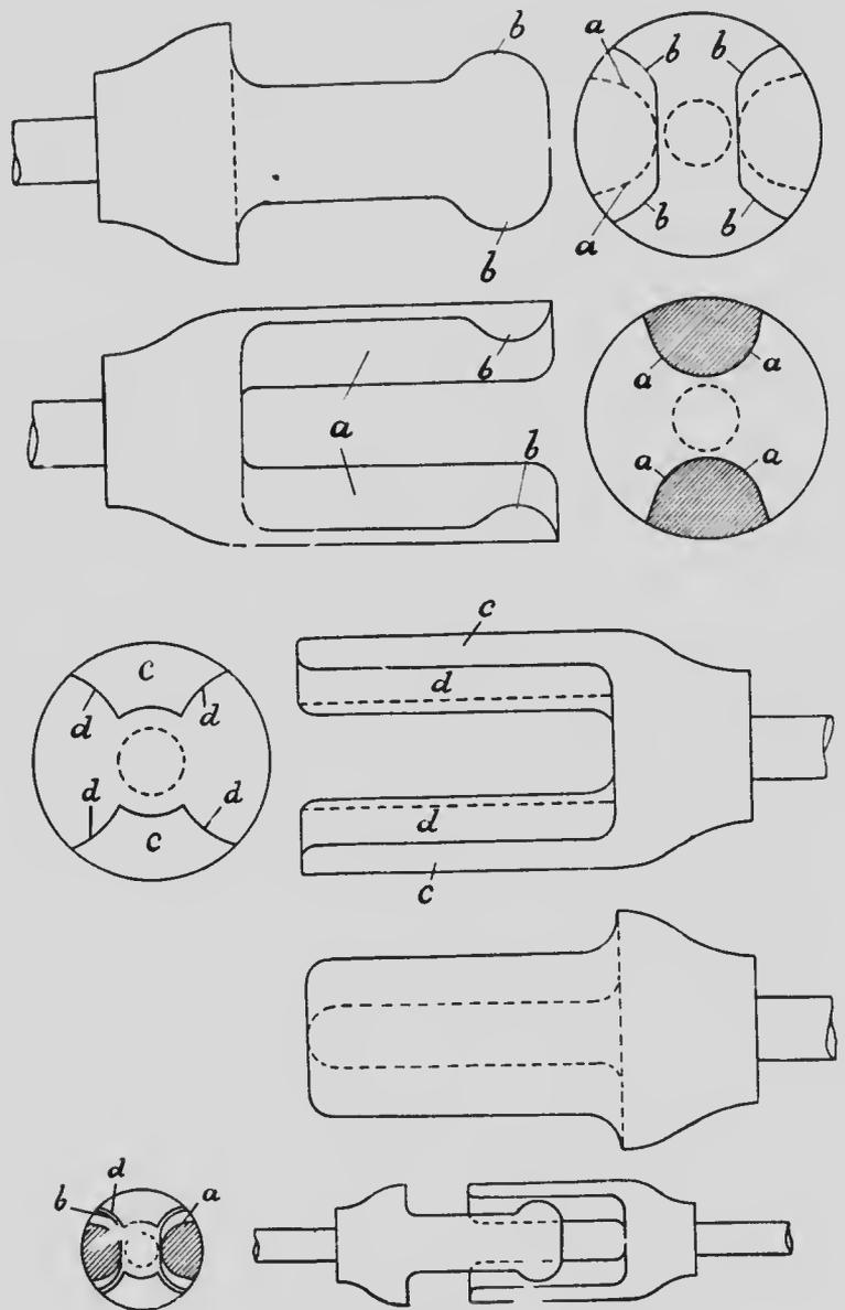
FIG. 120—Coupling to A. Körner's Peat Conveyor.
