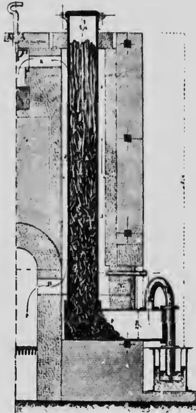
FIG. 211—Riché Gas-producer.
