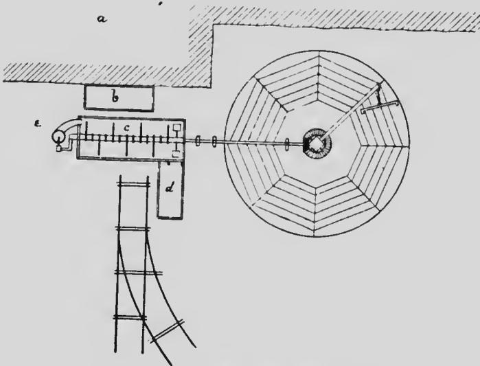
FIG. 32—General arrangements at a small Peat Plant.
