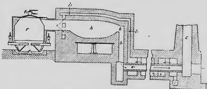
FIG. 196—Reverberatory Furnace, Fired with Producer-gas.
