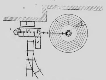
FIG. 32-General arrangements at a small Peat Plant,
