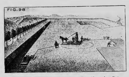
FIG. 98—General arrangement at a Dolberg Peat Plant with a one horse Peat Machine (in a drained bog).
