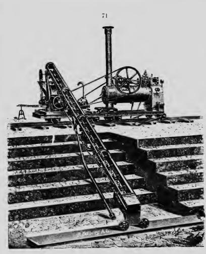
FIG. 68-R. Dolberg's Peat Plant with side elevator.
