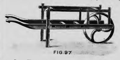
FIG. 97-Wheelbarrow for transport of Peat Pallets to drying field.
