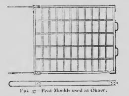
The peat porridge is <sup>1</sup> led at the bin on a train of 12 cars, which hanled to the drying field <sup>+</sup> vo horses attended by a man and a boy, w also attend to the loadit <sup>-</sup> Each car contains enough material to fill the moulds. Since the length of two cars is equal to that of three moulds, the train, when first brought up to the moulds, discharges only every other c it is then moved forward a distance equal to its own length, and then c charges the remaining full cars.
