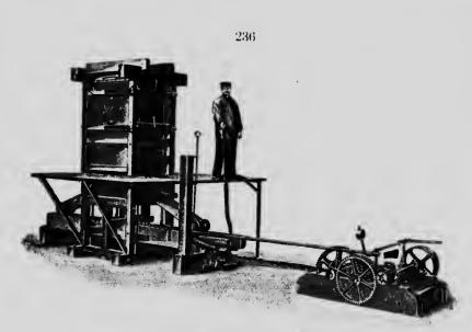
FIG. 225-Moss Litter Press for Motor-power.
