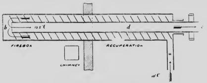
FIG. 171-Theoretical working of a Wet Carbonizing Oven.
