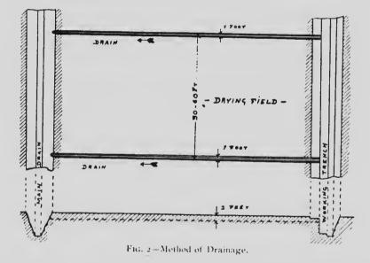
The surface of the bog is divided into squares, each of which generally is worked by two men, one man cutting the peat and placing it on the edge of the working trench, and the other loading it by hand or with a pitch fork on a wheel barrow or truck and transporting and laying it out on the drying field. In certain localities where lumber is fairly cheap special drying sheds or racks are sometimes used. (See pages 31–33). The area of the drying
