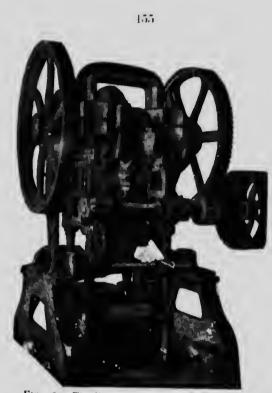
FIG. 169-The Dobson Peat Briquetting Press.
