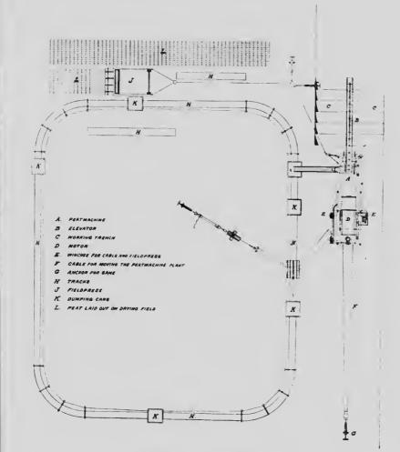
FIG. 114—Anrep Svedala Peat Plant with cable transportation on round track and fieldpress.
