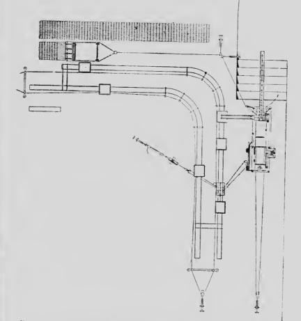
FIG. 116—Anrep Svedala Peat Plant with cable transportation on parallel tracks and field press.
