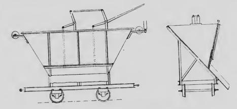
FIG. 46- Car for transport of pulped Peat at West Torup, Sweden,
