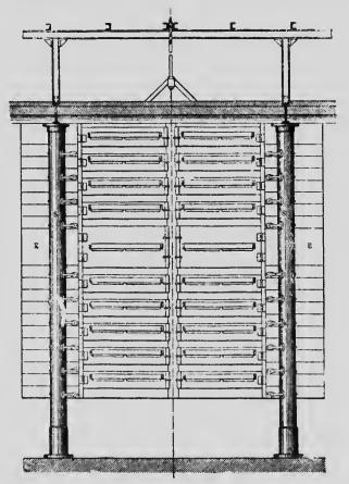
FIG, 146-Steam plate Drier (side view)
