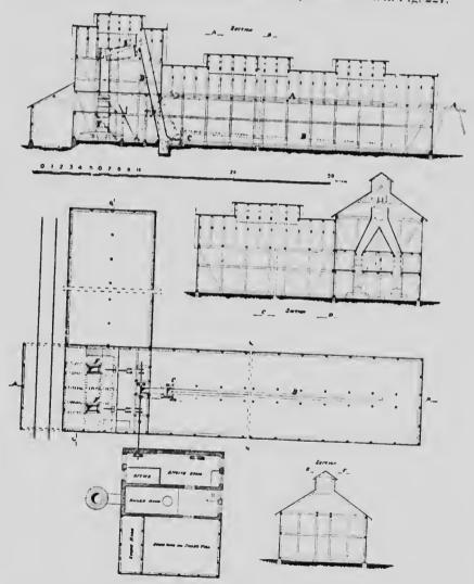
FIG. 228-Moss Litter Plant with Two Presses.
