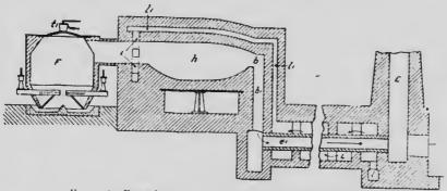
FIG. 196-Reverberatory Furnace, Fired with Producer-gas.
