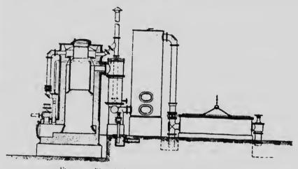
FIG. 203-Pintsch Gas-producer for Bituminous Fuels,
