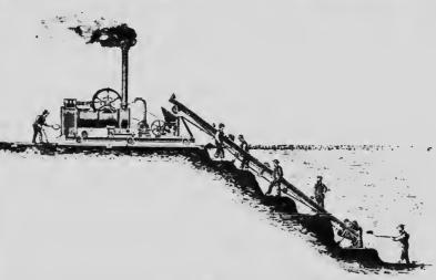
FIG. 69-R. Dolberg's Peat Plant with end elevator.
