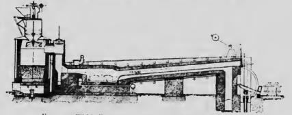
FIG. 195-Bildt's Producer combined with Re-heating Furnace.
