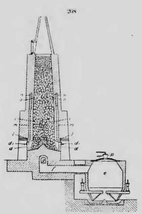
Fig. 198-Lime Kiln Fired with Producer-gas.
