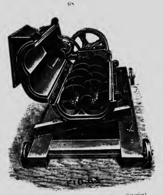
FIG. 63-R. Dolberg's Peat Machine No. 1a (interior).
