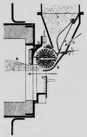
FIG. 192-Schwa: izkopf's Powder-firing Apparatus.
