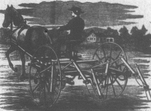
Experience has demonstrated the fact that a good HAY TEDDER that will thoroughly spread long, heavy grass, taking it up from the bottom, tossing it gently into the air, and leaving it upon the ground in a light, feecy condition, enables the farmer to take advantage of fair weather, and at least twice the quantity of hay can be secured, in better condition, than when allowed to remain in the swath.
