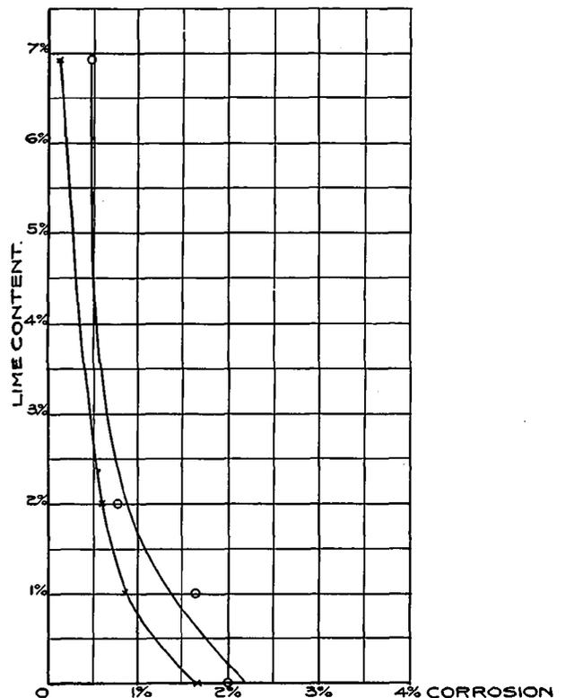
VARIATION OF CORROSION WITH PERCENTAGE OF HYDRATED LIME
