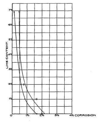
VARIATION OF CORROSION WITH PERCENTAGE OF HYDRATED LIME PLAIN STEEL-O. COPPER ALLOY-X
