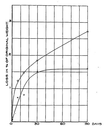
VARIATION OF CORROSION WITH TIME PLAIN STEEL-O, COPPER ALLOY-X
