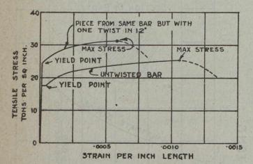
Fig. 2—Stress-strain Diagram for a 7/8 in. Diameter Bar, Before and After Twisting, Showing Respective Yield Points, Maximum Stress and Strain
