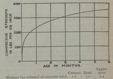
Fig. 3—Diagram showing Increase of Strength of Concrete with Age
