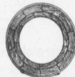
End View of Pipe and Coupling.
