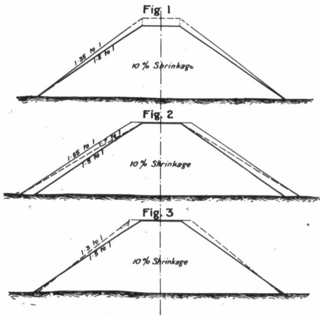
From these considerations it would appear reasonable to omit raising the fill above profile grade and applying side shrinkage only to make a full shoulder so as to carry the material required to make up to grade as bank settles.
