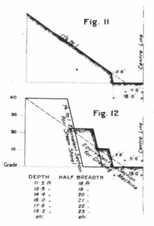
in Fig. 11, and in the cross-hatched section of Fig. 12. This increased the cut quantities slightly (as in Fig. 12 at ends of cut only), but the material being required in the fill, the overhaul only was increased. This cutting away of the toe of slope would be objectionable, if not impossible, in some instances, but here the banks caved back to a natural slope very quickly.
