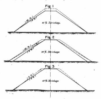
From these considerations it would appear reasonable to omit naising the fill above profile grade and applying side shrinkage only to make a full shoulder so as to carry the material required to make up to grade as bank settles.
