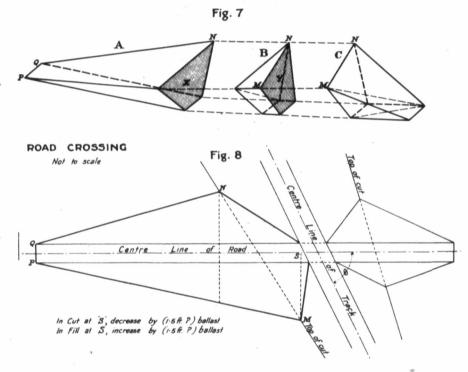
are the most important points to establish on the ground. P. and Q: should be laid out to give the requisite grade on road crossing between P.-Q. and the point S., otherwise the grade has to be steepened. Although a detail, this is often overlooked.
