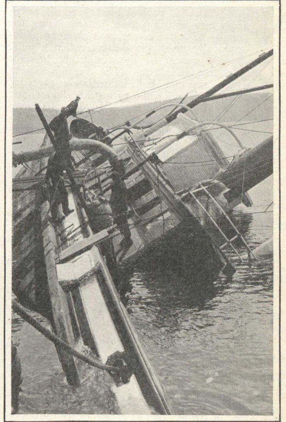
Raising the Dauntless, which ran ashore between Ladysmith and Chemainus. Especially pumping her out.
