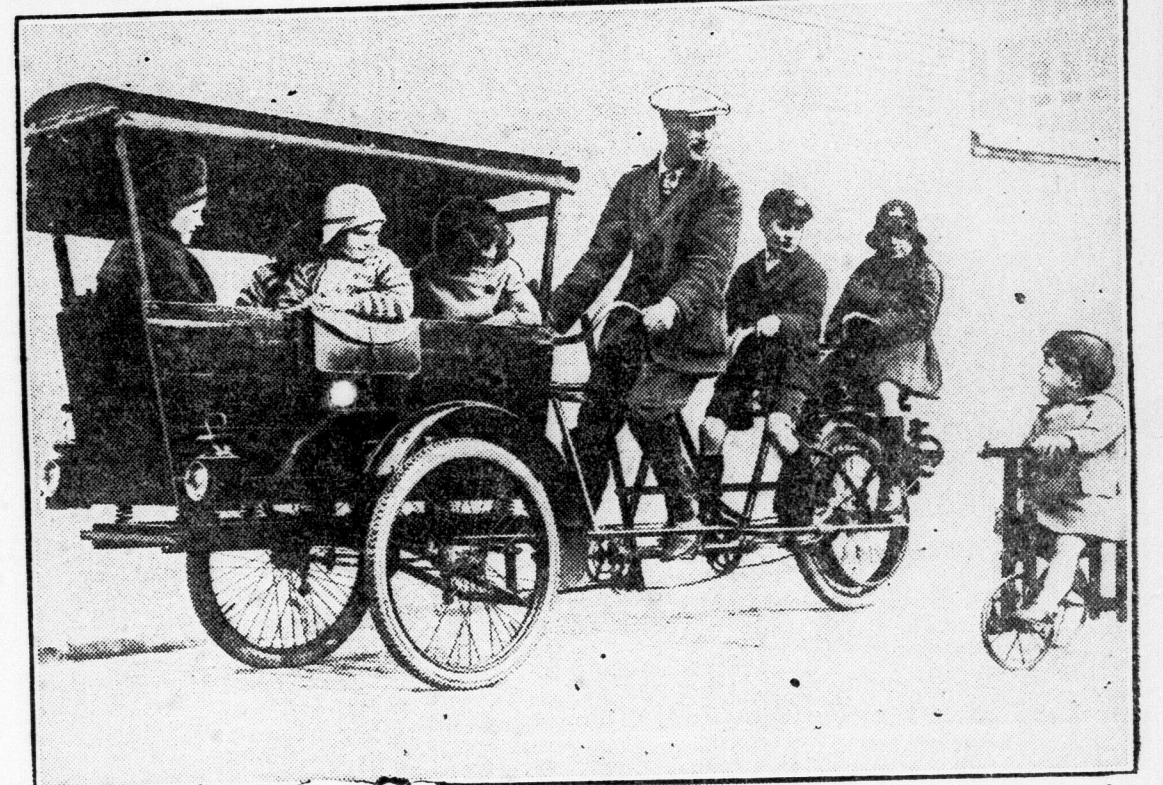
Family tricycle made by J. W. Wood of Highbury, England. The carrier is equipped with a detachable roof and side curtains. The affair is 12 feet long.
