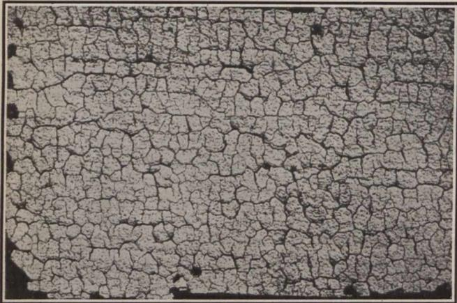
"Alligatoring."—Type of Decay Exhibited by Improperly Made Paint.
