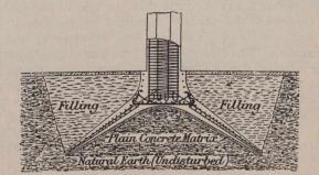
Sketch Showing Arrangement of Foundation in Place.
