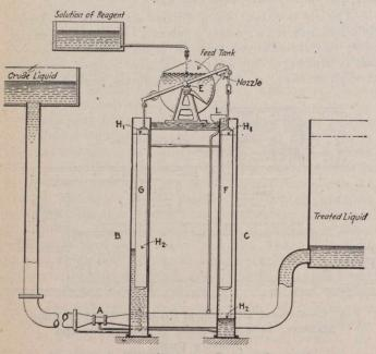
Diagram of the Tiltometer Dosing Apparatus.
