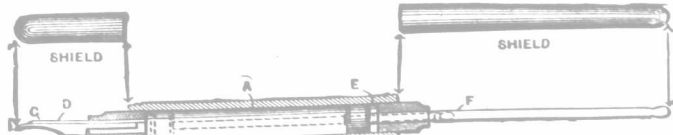
A, Barrel; B, Nozzle; C, Pen; D, Feed; E, Plunger; F, Rod.
