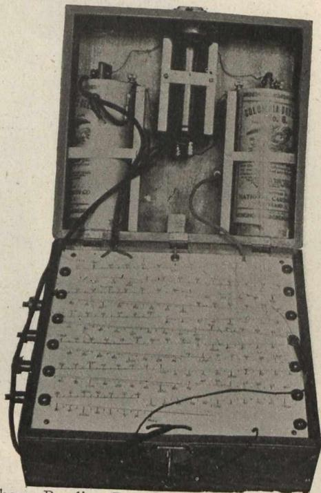
Telephone Reading Box to be Used With Pyrometer.
