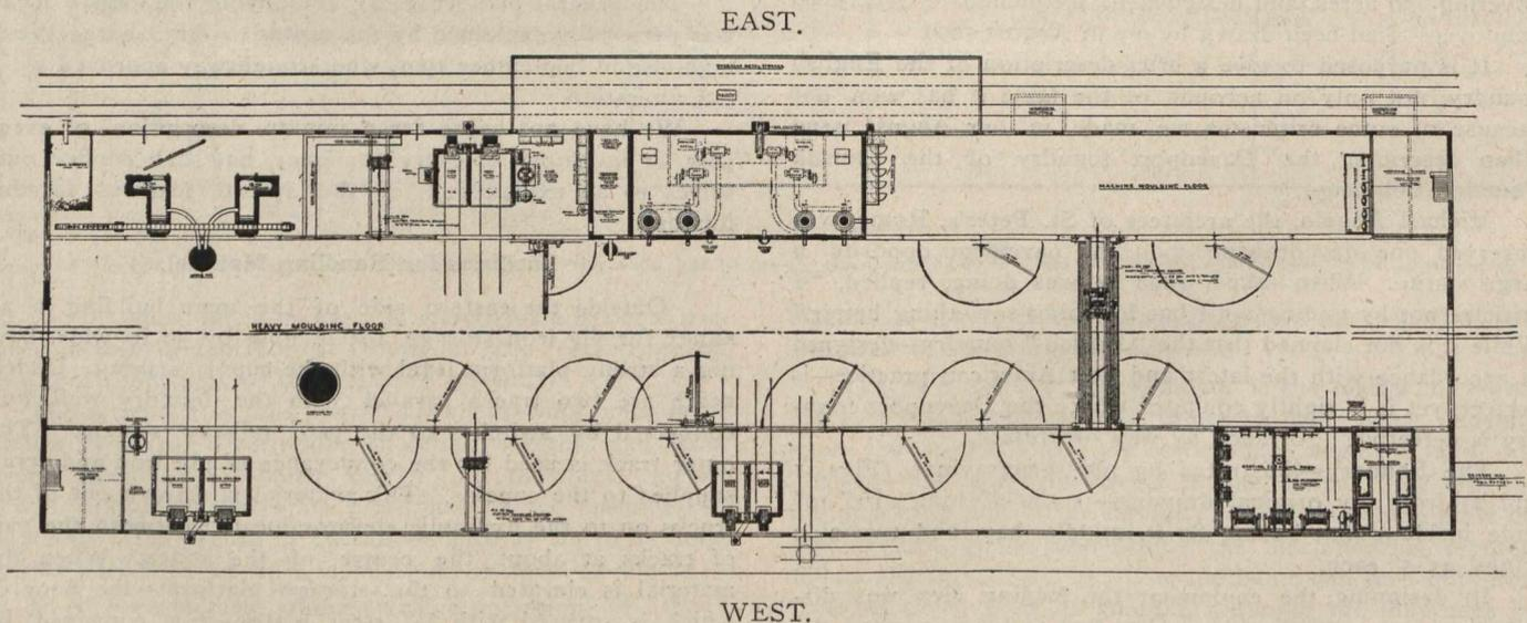
Fig. 2.—General Plan of British-Westinghouse Iron Foundry.
