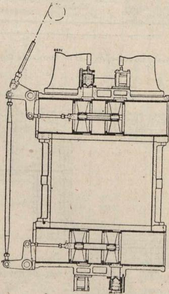
Fig. 3.—Section Through Air-Discharge Valves.
