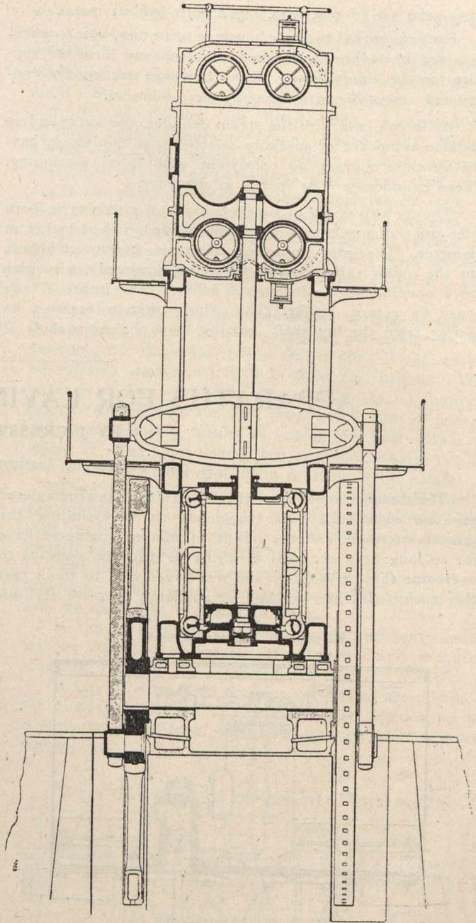
Fig. 2.—Vertical Section Through Blowing Engine.
