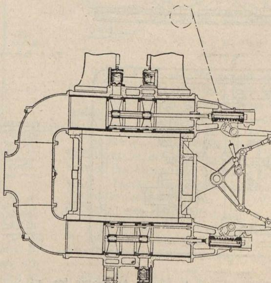
Fig. 4.—Section Through Air-Inlet Valves.
