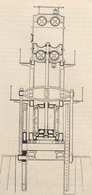
Fig. 2 .- Vertical Section Through Blowing Engine.
