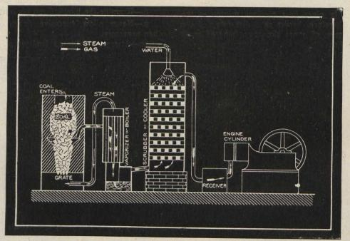
Diagram of Suction Gas Producer Plant and Engine.
