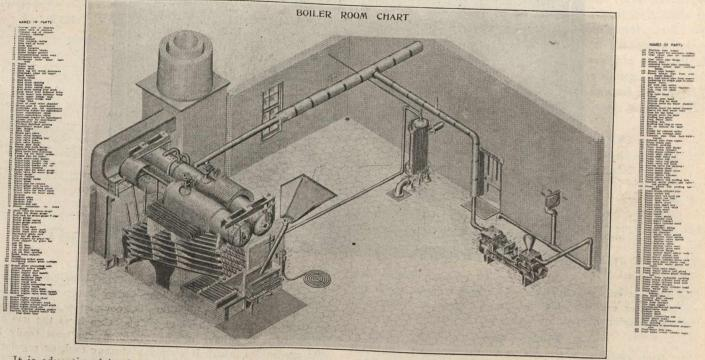
It is educational in that, with it, the student will be able to learn of the construction and arrangement of the best type of boiler plant, and examine into the relations of the various parts, while the glossary gives the name of each piece and part that is shown.
