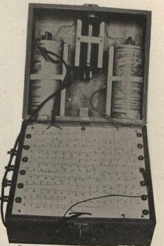
Telephone Reading Box to be Used With Pyrometer.
