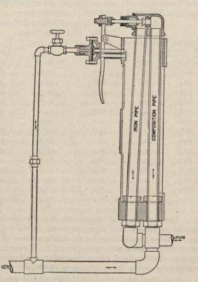
The force of expansion is used as in the regular Geipel Steam Trap to open and close the valve, and the pressure within the pipes is used to control the adjustment of the trap as it varies.
