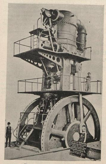
Fig. 1.-Morgan Blowing Engine.
