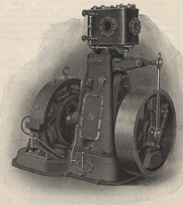
lubrication, etc., and the regulation is accomplished by means of a Rites' flywheel Inertia Governor, the speed variation being limited within 2% of full load, and no load.
