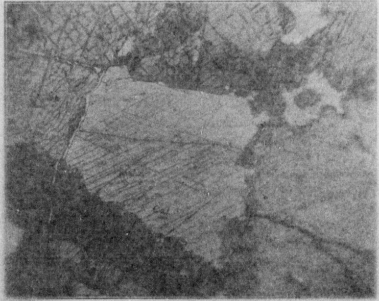
A. Micrograph showing primary calcite in matrix. The angular calcite grains are surrounded by a zone which shows a darker reaction than the matrix. Magnification, x 175. (See page 133)
