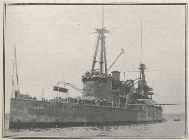
New Zealand's Battleship Anchored in Esquimalt Harbour, B.C., July 25. This New Imperial Warship is 555 Feet Long, With an 80-foot Beam, and a Displacement of 18,800 Tons.
