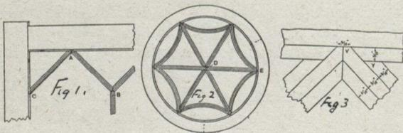
dimensions on the bars are given as 3-16 for the glass rabbets and 3-16 for the tongue of the bar. It is a fact that when the tongue is made thinner than 3-16 it is extremely difficult to brad them together in some of the joints without their splitting and spoiling the work.
