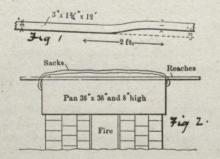
bender to do, that is, carefully protect the outside of his stock in bending with an iron strap, because he hasn't the regulation bending equipment. It is well, however, to keep it in mind and to strive wherever practical to give protection and reinforcement to the outside or at least have stops to the ends of the stick to prevent any chance for it to lengthen.
