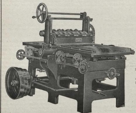
Feeds from 15 to 45 feet per minute. In feeding narrow stock through a 24-inch machine, for instance 4-inch stock, and feeding four pieces at the same time, the capacity at the end of the 10 hour day on the slowest feed would be 36,000 feet, and on the highest feed 108,000 feet.
