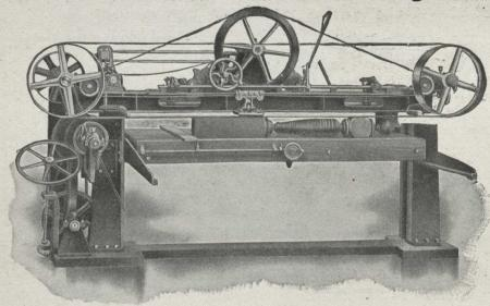
Takes either veneered or solid stock direct from the press and finishes without any hand work ready for the varnish room. The Variable Speed of pressure shoe prevents blistering or burning of stock. Owing to the open end the operator can sand material double the length of the table and can sand out any flaw in stock without reducing the thickness of edge. Operator has full control of all adjustments while machine is in operation.
