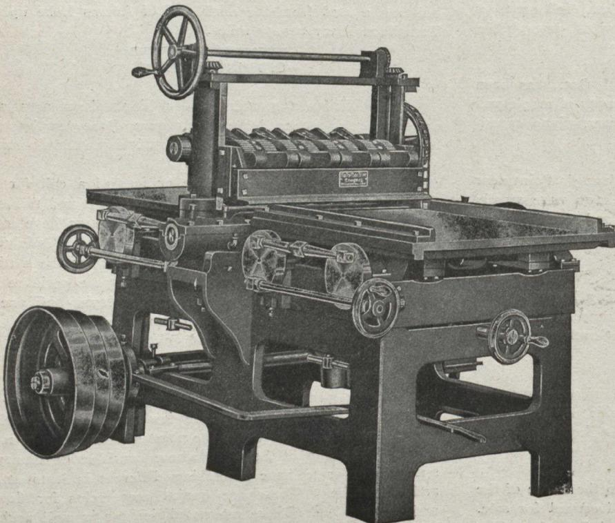
Feeds from 15 to 45 feet per minute. In feeding narrow stock through a 24-inch machine, for instance 4-inch stock, and feeding four pieces at the same time, the capacity at the end of the 10 hour day on the slowest feed would be 36,000 feet, and on the highest feed 108,000 feet.
