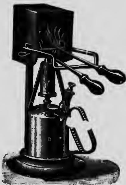
FIG. 217. — Automatic petroleum furnace and protecting hood for heating firing irons.
