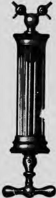
FIG. 228.—Double-acting syringe.
