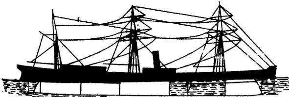
Fig. 5.—High Bulkheads. Two Holds Full. Vessel Floats.
