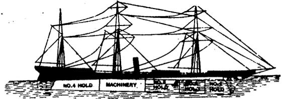
Bulkheads in Ships.—Fig. 1.—Bulkheads Stopped Too Low. Fig. 2.—Leak in No. 1 or No. 2 Hold. Vessel Goes Down.
