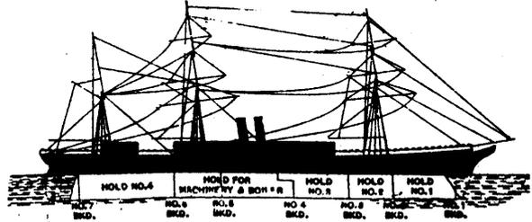
Fig. 6.—Water-Line Bulkheads. Common Arrangement.
