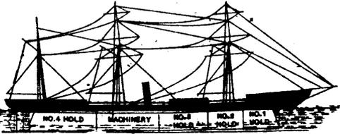
Fig. 3.—No Bulkheads. Result of a Leak. Vessel Floats.
