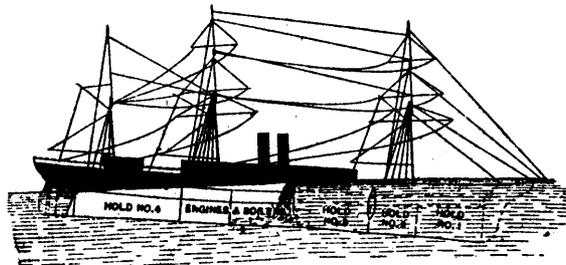
Bulkheads in Ships.—Fig. 7.—Result of Collision with Water-Line Bulkheads.
