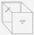
Before attempting the making of pictures it is of the utmost importance that you fully understand your camera and its equipment. A camera in its simplest form would be a simple box, made light tight, with a lens at one end and a means for supporting a plate or film inside the box at the other end, as illustrated in the accompanying diagram.
