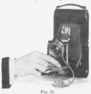
The front can be moved to the right or left (up and down when Kodak is placed on its side for horizontal exposure) by loosening thumb screw directly under the shutter as shown in Fig II., and sliding front in either direction to the desired position. Lock in position by tightening thumb screw. When through using, reverse the operation shown in Fig. II., and slide back to the center and lock in position.
