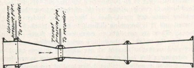
Fig. 9 Longitudinal section of Venturi Meter
