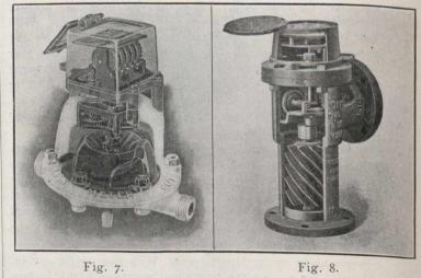
the piston for the former, but when the disc and disc chamber of the disc meter become worn the meter's usefulness is ended.
