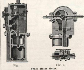
to "stick up" or stop, and when not registering when water is being passed through it should give some outward indication of the fact; and, finally, should be incapable of passing water backwards.
