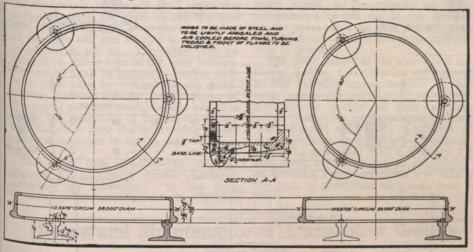
Fig. 1, Wheel Circumference Measure Test Rings for 33 and 36 in. Wheels.
