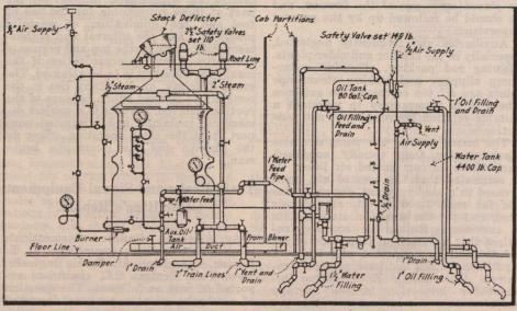
Assembled Installation of Oil-Fired Heating Equipment.
