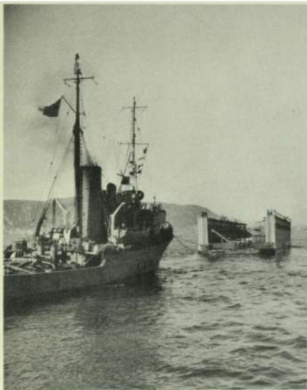
Bassin de raboub flottant remorqué vers St. John's. Septembre 1943. Floating drydock being towed into St. John's, September, 1943.
