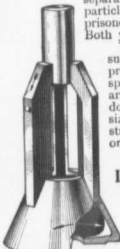
Dirt-arrester chamber with part of side bushes away to show — the impurities are collected.
